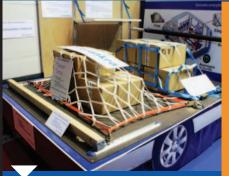
Light vehicle load restraint is steadily creeping up the enforcement agenda in France, which means the UK could soon follow. Swedish outfit **Forankra** showcased webbing-based cargo nets specifically for car-derived, compact and large panel vans. Attached to existing load restraint points in the body floor, the nets can be tightened down around the base, using an integrated ratchet strap. The largest net for 3.5-tonners measures 1.3 x 2.2m.
