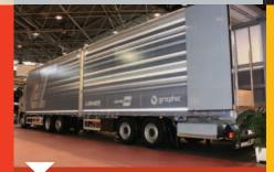
This maximum volume Libner 'Eurolib' concept is based around a New Actros 2542 6x2 wagon and Frejat tandemaxle drawbar trailer. It features a telescopic hydraulic drawbar coupling that facilitates rapid through-cargo loading, via a hinged front bulkhead on the trailer.
