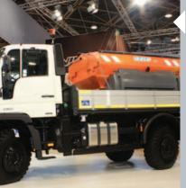
This U500 Unimog, with Arvel Snow-Tec plough and demountable gritter pack, features all-wheel-drive steering, which is now available as a factory option. Command electronics and hydrostatic steering components have been developed and provided by UK Unimog specialist South Cave Tractors. Steering rear-axle has hydro-mechanical locking mechanism and is derived from existing driven front-axle. The system uses electronic potentiometers to ensure correct steering angles, front and rear.
