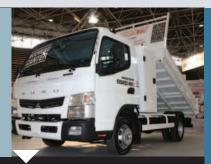
The new **Mitsubishi Fuso Canter** arrives in the UK in early 2012, with 3.5 and 7.5-tonnes options, and a 4x4 to follow. All are powered by the latest 3-litre engine, rated between 130 and 175bhp, along with optional Duonic dual-clutch automatic transmission, in place of a five-speed manual.
